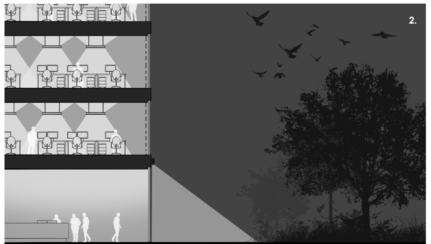
2. Strategically located internal illumination, carefully detailed glazing facades and good optical control on for external lighting can help prevent light trespass into green areas spaces and birdstrike.
